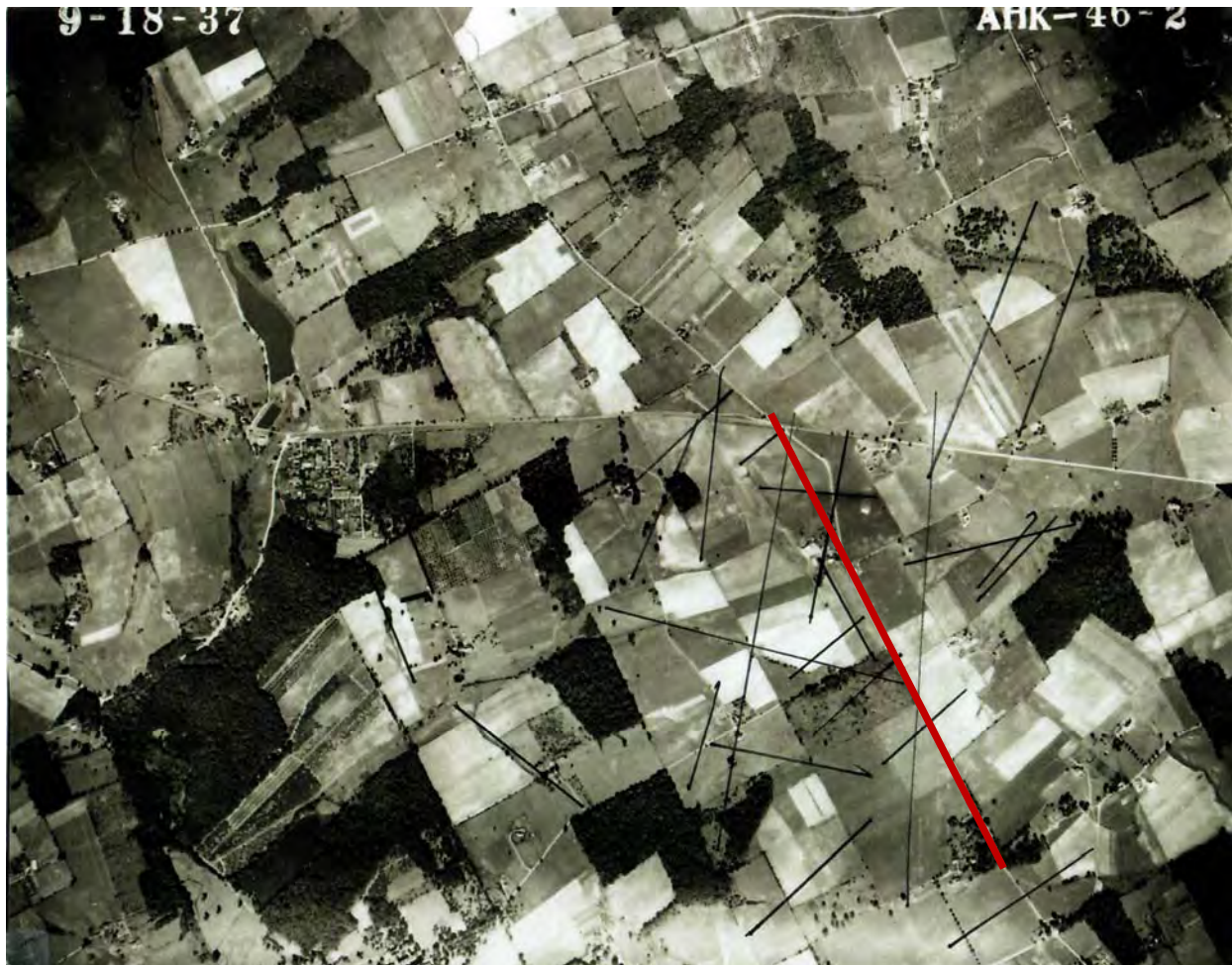
Figure 3. Fracture Trace Analysis (HDD S3-0541 approximate location shown as red line)
