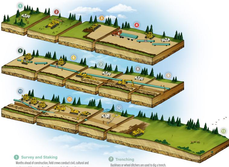
environmental surveys along the proposed pipeline route, or right-of-way. A final route is then selected and marked with stakes.
