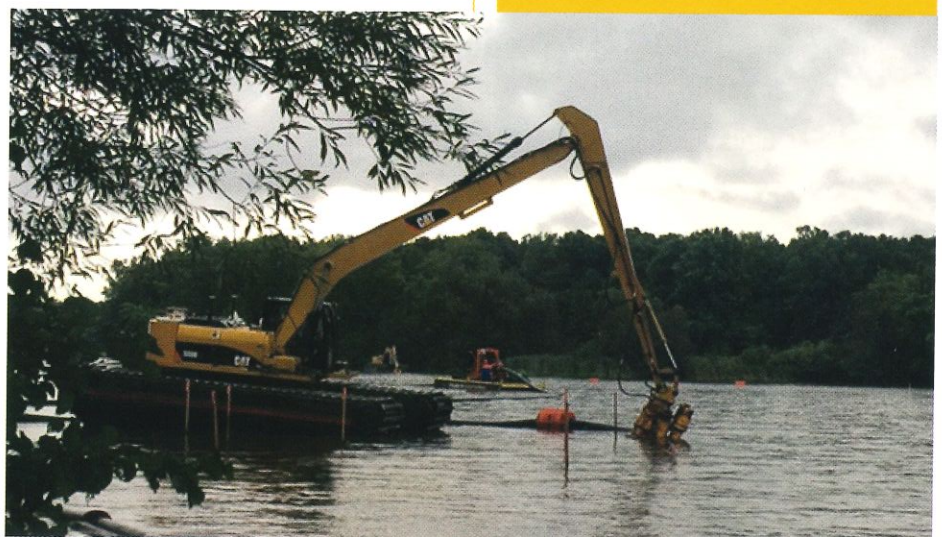
Dredging equipment is utilized to contain and remediate an oil spill near the Kalamazoo River. Photo credit: Justin Ritter.
