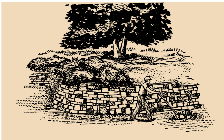
Figure 15. Attractive retaining walls can be used to limit the size of fill and cut slopes, increasing the size of a tree's protection zone.
