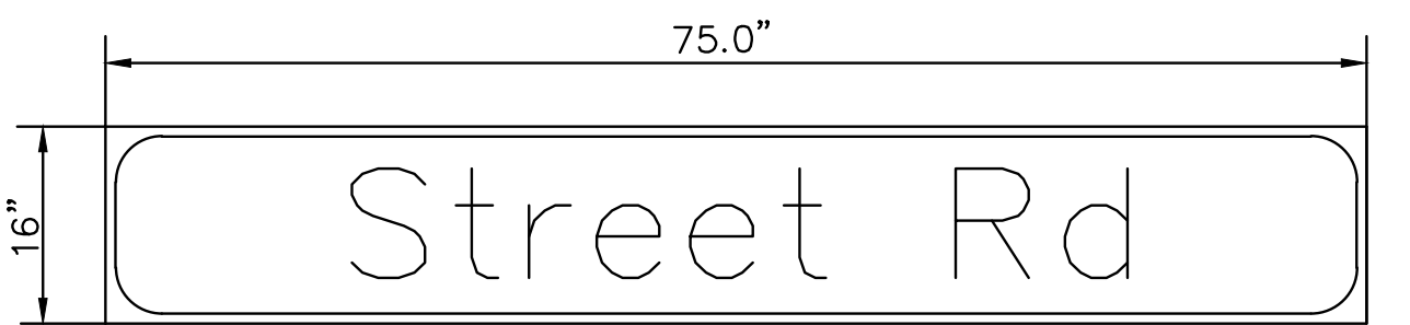
SIGN F DETAIL 8.0" UPPER CASE 6.0" LOWER CASE CLEARVIEW
