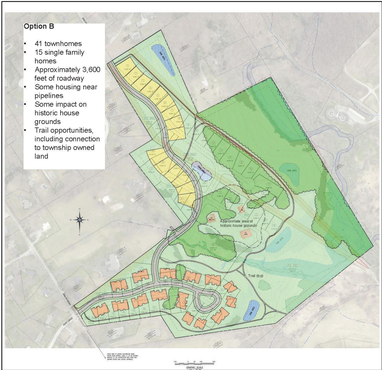
CCPC Alternative Sketch Plan – Option B (Base drawing from sketch plan, prepared by D.L. Howell & Associates, Inc., dated 11/10/2020)
